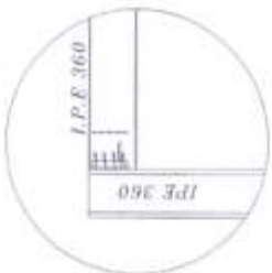
DETAIL 1 TH. OF PL. = 10mm BOLTS M18 (8.8)
