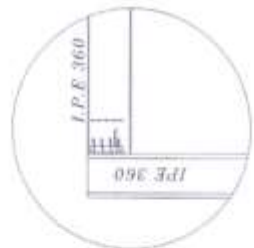
DETAIL 1 TH. OF PL. = 10mm BOLTS M18 (8.8)
